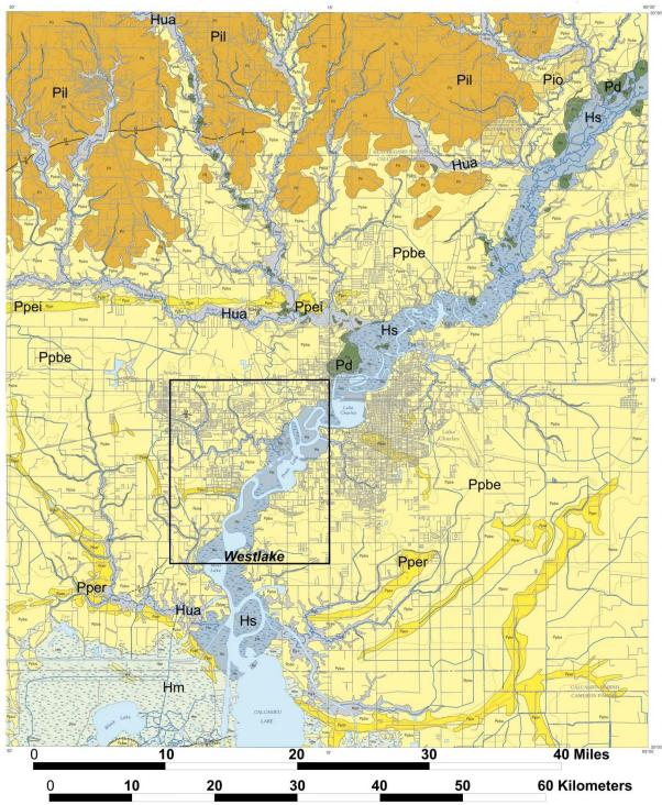
2. Surface geology of the area encompassing the Westlake 7.5-minute quadrangle (excerpted and adapted from Heinrich et al., 2002). (Pil, Lissie Alloformation, undifferentiated; Pio, Oakdale alloformation; Ppbe, Beaumont Alloformation; Ppei, Relict Pleistocene barrier ridge (Houston ridge); Pper, Relict Pleistocene ridges; Pd, Deweyville Allogroup, undifferentiated; Hm, Mermentau Alloformation; Hs, Small river deposits, undifferentiated; Hua, Holocene undifferentiated alluvium).
