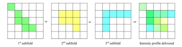
Figure 1. Intensity profile delivered from MLC sequence
