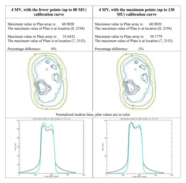
Figure 33. Comparison based on calibration curves used (4 MV)
