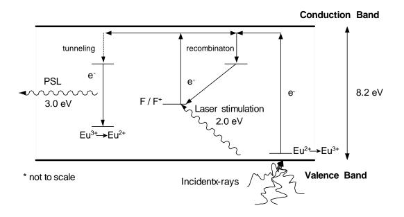
**Figure 5. PSL mechanism in BaFBr:**Eu<sup>2+</sup> (for purposes of illustration e<sup>-</sup> propagation goes from right to left)
