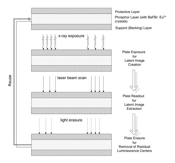
Figure 7. Readout cycle
