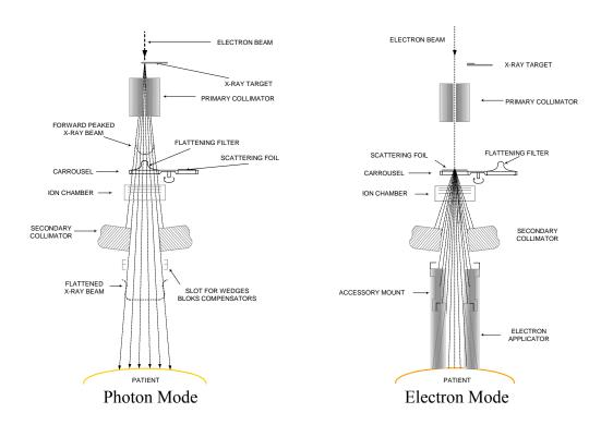
Figure 4. Accelerator head
