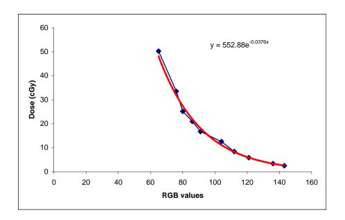
Figure 28. Calibration curve (4 MV)
