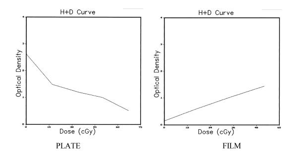
Figure 24. Example of calibration curve done with RIT113 v. 3.14
