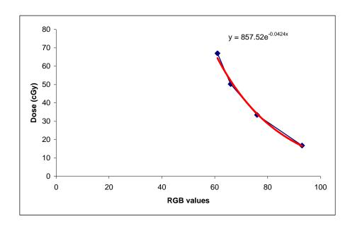
Figure 26. Plate calibration curve (4 MV), trendline in red
