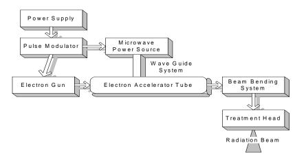
Figure 3. Block diagram of typical medical LINAC
