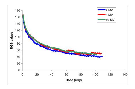
Graph below shows comparison of the calibration curves for three different energies using the data points calculated with the exponential equation for the maximum number of monitor units delivered, these are the curves actually used for CR plate's calibration in developed IMRT analysis program.
