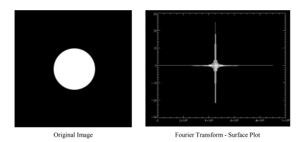
Figure 46. Fourier transform of a uniform disk
